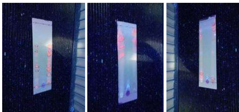
Figure 1. Thin Layer Chromatography (TLC) Analysis Determination of Solvents or Solvent Mixtures
