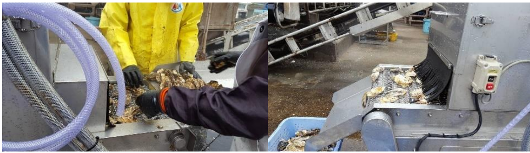
Figure 10. Oyster washing using a pressure machine
